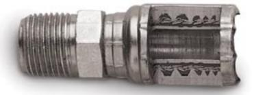
The advanced design of the MegaCrimp tooth profile shown above "bites the wire" for better coupling retention unlike the competitive crimp shown below that relies on the compression of the rubber.
