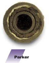
The "polygon effect" is even more dramatic when the couplings are crimped without the hose!
